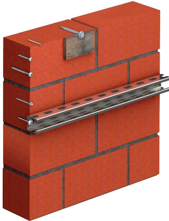
Screw anchors MMS, MMS-ST and HMS-KS from OBO Bettermann offer optimum fastening options in solid masonry types. The various dimensions and head shapes provide installation options for the different routing components. The screw anchors ties are screwed directly into the drill hole. There is no need for an additional anchor. No spreading forces develop and mounting near masonry edges is not required. You can find detailed information in the corresponding approvals.
