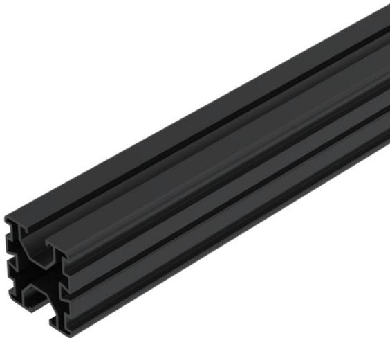
Support profile to mount photovoltaic modules on flat and pitched roofs. Flat roof mounting in combination with UniBase universal stand and STK and STL short and long supports. Lockable fastening of the profile on the stand with UniBase AMP adapter. Pitched roof mounting in combination with universal DHU roof hook. Lockable fastening of the profile on roof hooks. Screwable connection of multiple support profiles with LV 45 straight connectors and KV 45 cross-connectors.
