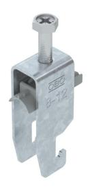
Clamp clip with U-foot, plastic pressure sleeve made of polypropylene. For vertical and horizontal mounting of 2 single cables on a C-profile rail. For slot width 18–22 mm. With 1-start screw thread on pressure sleeve, universal hexagonal screw head WAF10, with slot and cross recess. Suitable for assembly indoors and outdoors. Multiple cables should be separated by double sleeves. We recommend the use of a counter-sleeve.
