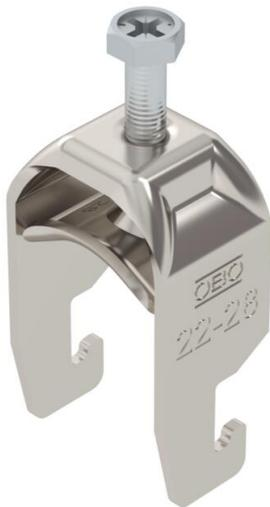
Clamp clip with U-foot, metal pressure sleeve with rounded edges to protect the cable. For vertical and horizontal mounting of 1 single cable on a C-profile rail. For slot width 18–22 mm. With 1-start screw thread on pressure sleeve, universal hexagonal screw head WAF10, with slot and cross recess. Suitable for assembly indoors and outdoors. We recommend the use of a counter-sleeve.
