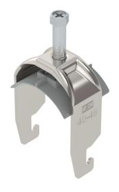
Clamp clip with U-foot, plastic pressure sleeve made of polypropylene. For vertical and horizontal mounting of 1 single cable on a C-profile rail. For slot width 18–22 mm. With 1-start screw thread on pressure sleeve, universal hexagonal screw head WAF10, with slot and cross recess. Suitable for assembly indoors and outdoors. We recommend the use of a counter-sleeve.
