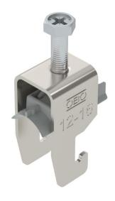
Clamp clip with U-foot, plastic pressure sleeve made of polypropylene. For vertical and horizontal mounting of 1 single cable on a C-profile rail. For slot width 18–22 mm. With 1-start screw thread on pressure sleeve, universal hexagonal screw head WAF10, with slot and cross recess. Suitable for assembly indoors and outdoors. We recommend the use of a counter-sleeve.
