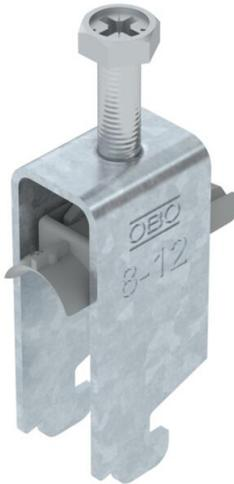
Clamp clip with N-foot, plastic pressure sleeve made of polypropylene. For vertical and horizontal mounting of 2 single cables on a C-profile rail. For slot width 11–12 mm With 1-start screw thread on pressure sleeve, universal hexagonal screw head WAF10, with slot and cross recess. Suitable for assembly indoors and outdoors. Multiple cables should be separated by double sleeves. We recommend the use of a counter-sleeve.
