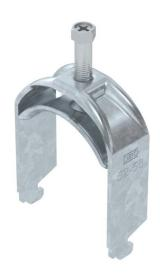
Clamp clip with N-foot, metal pressure sleeve with rounded edges to protect the cable. For vertical and horizontal mounting of 1 single cable on a C-profile rail. For slot width 11–12 mm With 1-start screw thread on pressure sleeve, universal hexagonal screw head WAF10, with slot and cross recess. Suitable for assembly indoors and outdoors. We recommend the use of a counter-sleeve.
