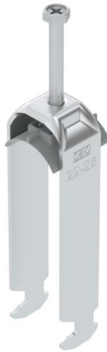
Clamp clip with hammerhead foot, plastic pressure sleeve made of polypropylene. For vertical and horizontal mounting of 3 single cables on a C-profile rail. For a slot width 16–17 mm. With 1-start screw thread on pressure sleeve, universal hexagonal screw head WAF10, with slot and cross recess. Suitable for assembly indoors and outdoors. Multiple cables should be separated by double sleeves. We recommend the use of a counter-sleeve.
