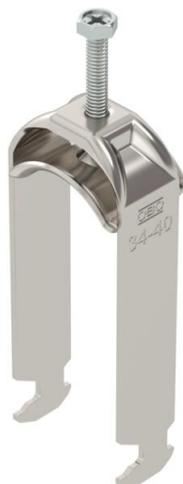
Clamp clip with hammerhead foot, metal pressure sleeve with rounded edges to protect the cable. For vertical and horizontal mounting of 2 single cables on a C-profile rail. For a slot width 16–17 mm. With 1-start screw thread on pressure sleeve, universal hexagonal screw head WAF10, with slot and cross recess. Suitable for assembly indoors and outdoors. Multiple cables should be separated by double sleeves. We recommend the use of a counter-sleeve.
