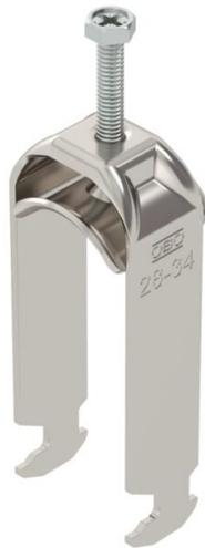
Clamp clip with hammerhead foot, metal pressure sleeve with rounded edges to protect the cable. For vertical and horizontal mounting of 2 single cables on a C-profile rail. For a slot width 16–17 mm. With 1-start screw thread on pressure sleeve, universal hexagonal screw head WAF10, with slot and cross recess. Suitable for assembly indoors and outdoors. Multiple cables should be separated by double sleeves. We recommend the use of a counter-sleeve.
