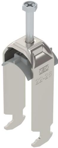
Clamp clip with hammerhead foot, plastic pressure sleeve made of polypropylene. For vertical and horizontal mounting of 2 single cables on a C-profile rail. For a slot width 16–17 mm. With 1-start screw thread on pressure sleeve, universal hexagonal screw head WAF10, with slot and cross recess. Suitable for assembly indoors and outdoors. Multiple cables should be separated by double sleeves. We recommend the use of a counter-sleeve.
