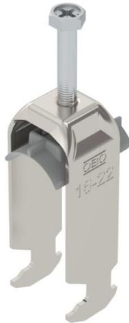
Clamp clip with hammerhead foot, plastic pressure sleeve made of polypropylene. For vertical and horizontal mounting of 2 single cables on a C-profile rail. For a slot width 16–17 mm. With 1-start screw thread on pressure sleeve, universal hexagonal screw head WAF10, with slot and cross recess. Suitable for assembly indoors and outdoors. Multiple cables should be separated by double sleeves. We recommend the use of a counter-sleeve.
