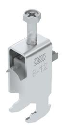
Clamp clip with hammerhead foot, plastic pressure sleeve made of polypropylene. For vertical and horizontal mounting of 2 single cables on a C-profile rail. For a slot width 16–17 mm. With 1-start screw thread on pressure sleeve, universal hexagonal screw head WAF10, with slot and cross recess. Suitable for assembly indoors and outdoors. Multiple cables should be separated by double sleeves. We recommend the use of a counter-sleeve.
