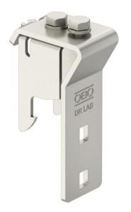
Spacer for stand-off mounting of covers on wide span cable trays and wide span cable ladders. Space height 35 mm, stainless steel 1.4301.
